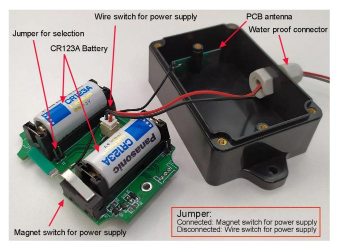
(When the alarm is over, **Both the switches** must be restored to the power-off state (that is, the magnetic steel sucks back the switch and the input line should be disconnected, otherwise the box cannot be completely powered off, and a small amount of power will continue to be consumed until both switches are off)
