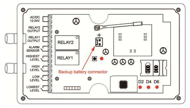
LED D2: SMS Receiver and Transmitter Status
